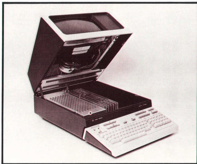
Fig. 1. Model 2640A Interactive Display Terminal operates in either character or page mode. Data transmission is compatible with EIA RS 232C and with Bell type 103 and 202 modems. Data rates from 110 to 2400 baud are selectable. Character code for data transmission is ASCII.
